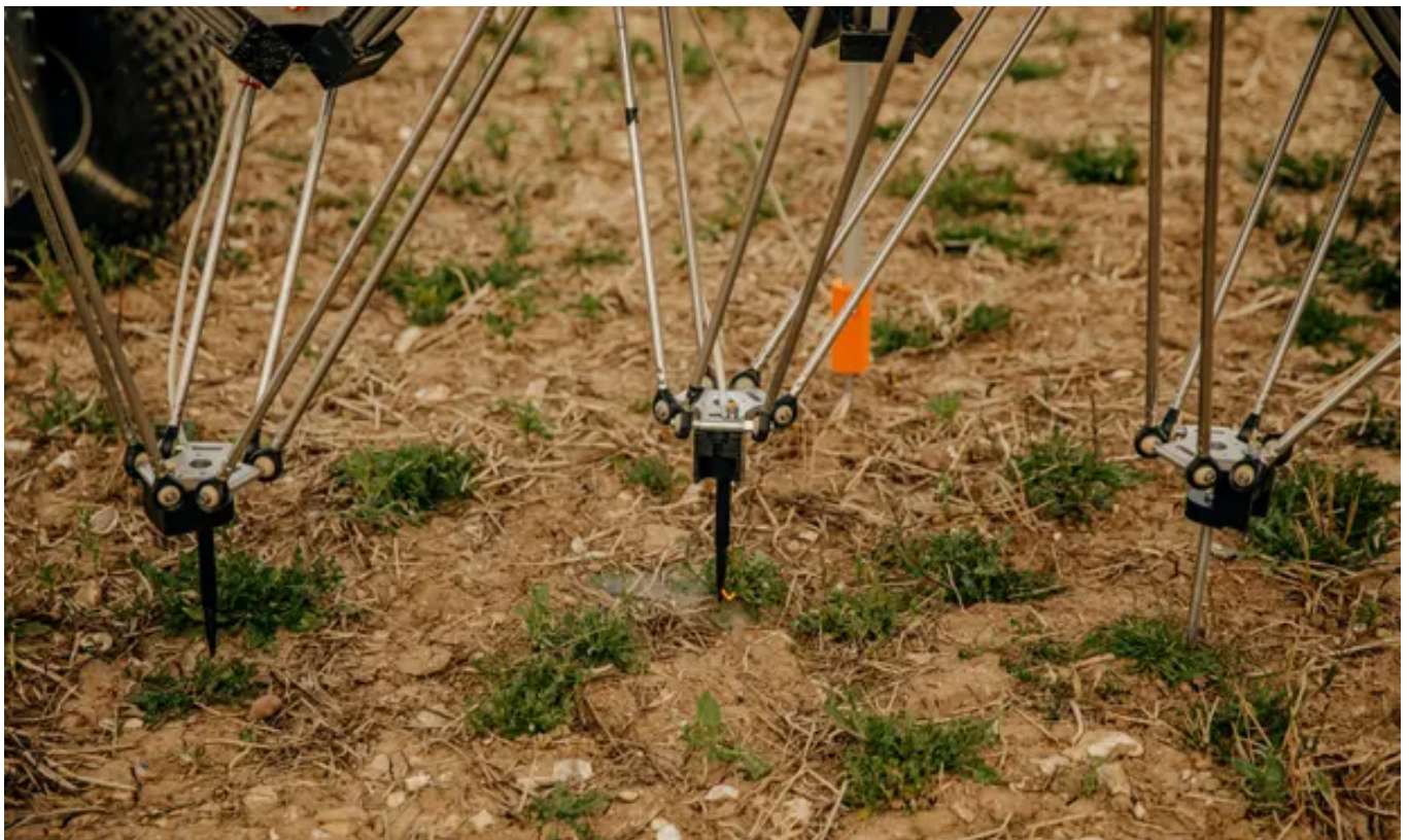
📹 Dick demonstrates its weedkilling electrode. Photograph: Peter Flude/The Guardian
